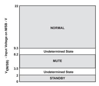
Figure 24. Standby, Mute, and Normal (On) Operating Conditions
