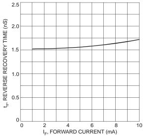
Fig. 4 Reverse Recovery Time vs. Forward Current
