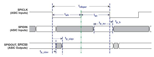
Figure 15. Flash Interface Timing
