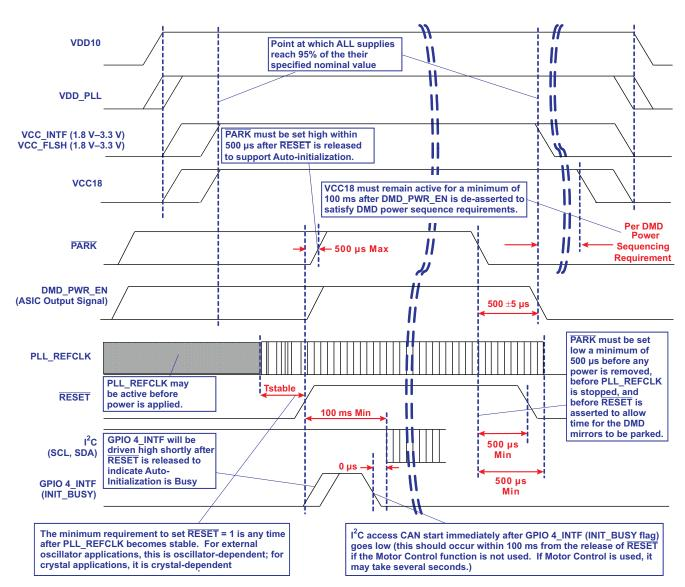
Figure 19. Power-Up/Down Timing
