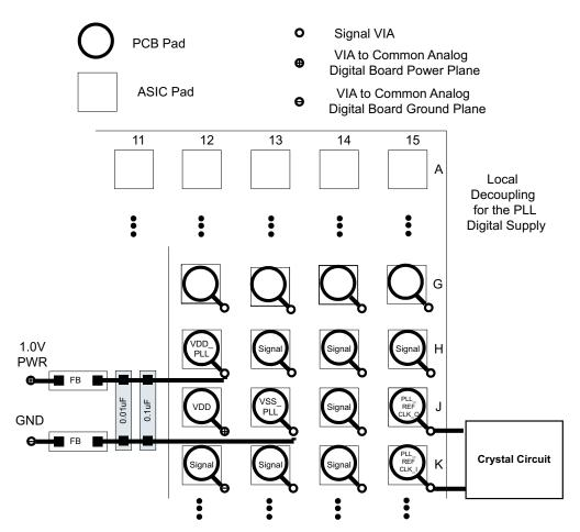
Figure 21. PLL Filter Layout
