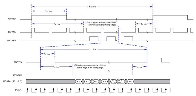
Figure 12. Parallel I/F Frame Timing
