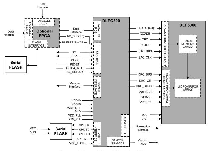
Figure 6. DLP3000 Chipset With Optional FPGA
