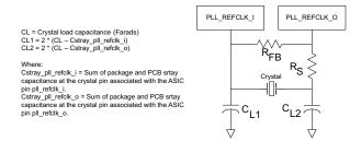
Figure 20. Recommended Crystal Oscillator Configuration
