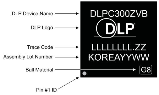
Figure 9. Device Marking
