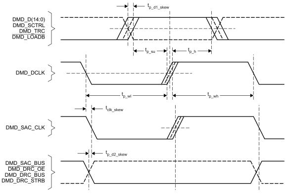
Figure 16. DMD Interface Timing
