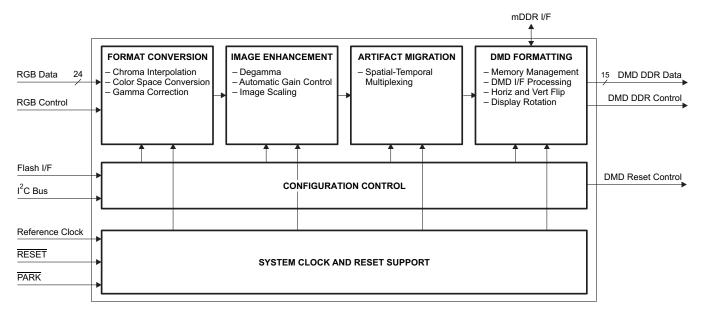
Figure 2. DLPC300 Functional Block Diagram
