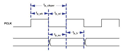
Figure 13. Parallel and BT.656 I/F General Timing
