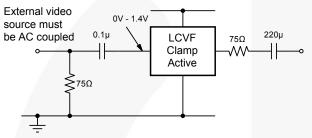
Figure 18. Biased SCART with AC-Coupled Outputs
