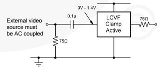
Figure 16. SCART with DC-Coupled Outputs
