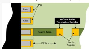
Figure 19. Recommended Resistor Placement
