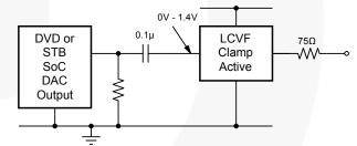
Figure 15. AC-Coupled Inputs, DC-Coupled Outputs
