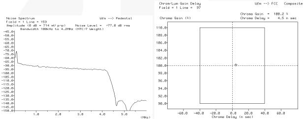
Figure 9. SNR vs Frequency Figure 10. Chroma/Luma Gain & Delay
