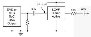
Figure 17. AC-Coupled Inputs and Outputs
