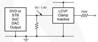
Figure 14. DC-Coupled Inputs and Outputs
