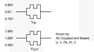
Figure 12. Typical Voltage Levels
