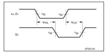
Waveform 2. Propagation Delay for Non-Inverting Outputs
