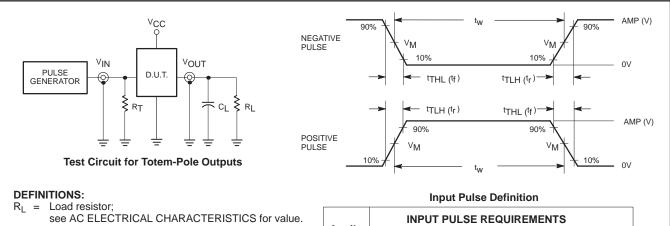
$C_L = Load$  capacitance includes jig and probe capacitance; see AC ELECTRICAL CHARACTERISTICS for value.
