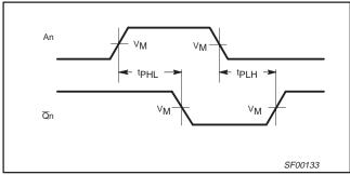
Waveform 1. Propagation Delay for Inverting Outputs
