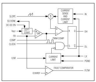
Figure 4. Step-Down Controller Block Diagram
