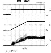
B: OUTPUT VOLTAGE, 2V/div C: INDUCTOR CURRENT, 1A/div
