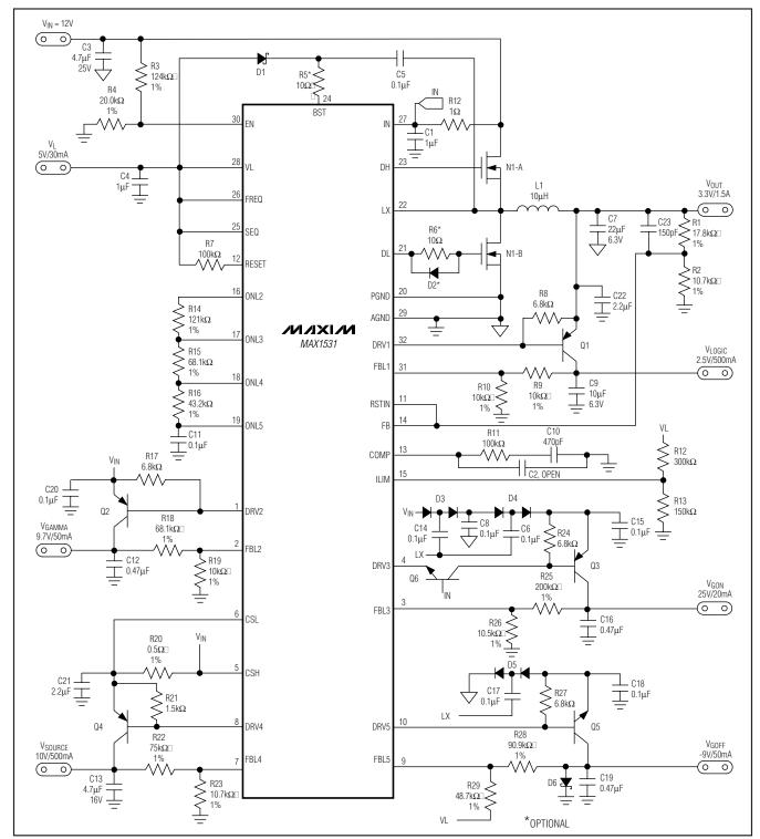
Figure 1. MAX1531 Standard Application Circuit
