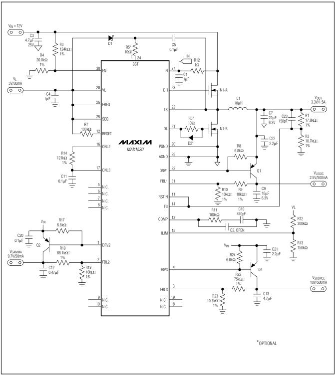
Figure 2. MAX1530 Standard Application Circuit
