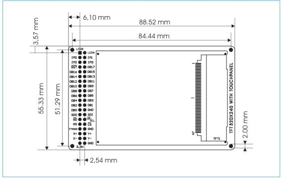
Figure 4: Dimensions of the TFT PROTO additional board
