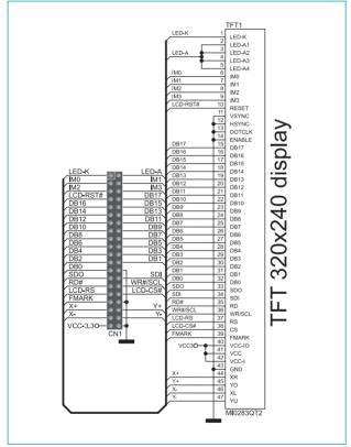
Figure 2: TFT PROTO additional board connection schematic
