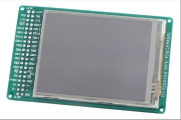
Figure 1: TFT PROTO additional board
