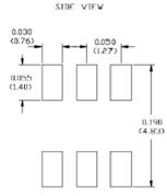
\* Dimensions are inches (millimeters) ±0.015 (0.38) unless otherwise specified.
