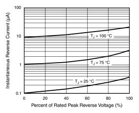
Figure 4. Typical Reverse Characteristics
