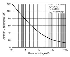
Figure 5. Typical Junction Capacitance Per Leg
