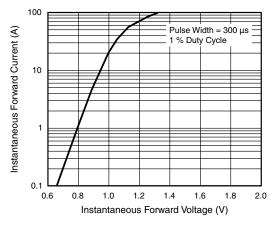
Figure 3. Typical Instantaneous Forward Characteristics
