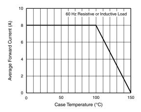
Figure 1. Forward Current Derating Curve
