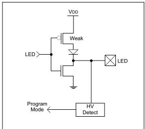
FIGURE 2-7: LCCOM/LCX/LCY/LCZ/ VSST PIN DIAGRAM
