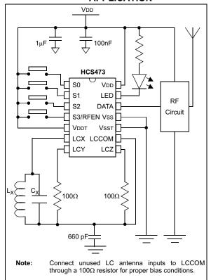
FIGURE 2-3: S0/S1/S2 PIN DIAGRAM
