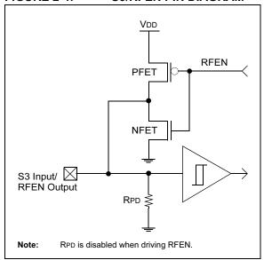
FIGURE 2-5: DATA PIN DIAGRAM
