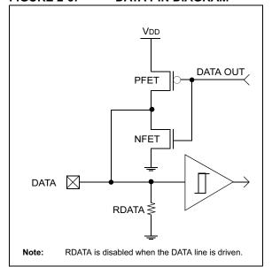
FIGURE 2-6: LED PIN DIAGRAM
