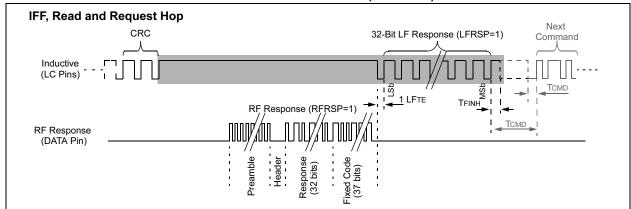
FIGURE 3-21: LF COMMUNICATION ANALOG DELAYS
