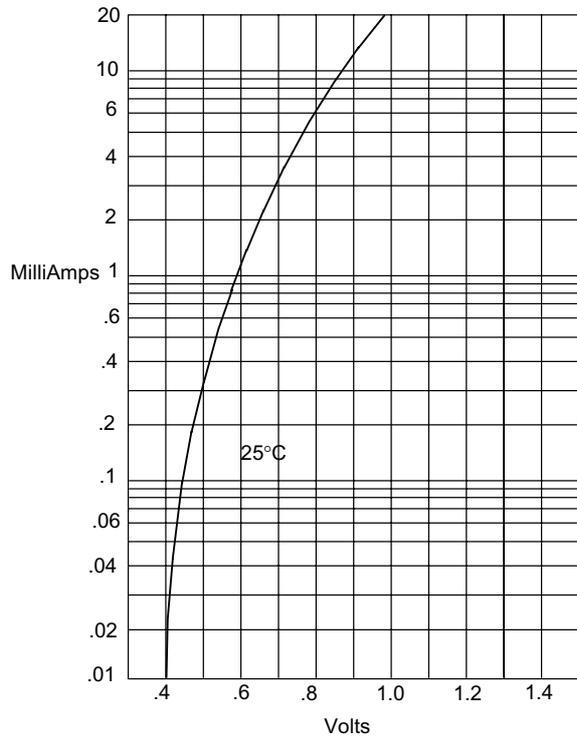
Instantaneous Forward Current - Amperes *versus*
