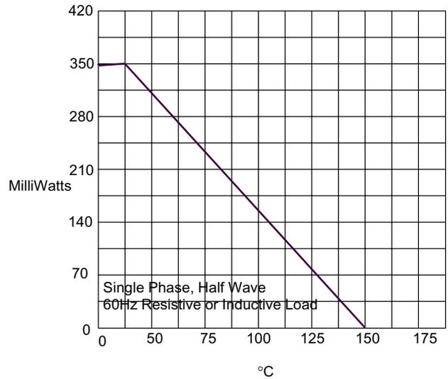
Admissible Power Dissipation - MilliWatts *versus*
