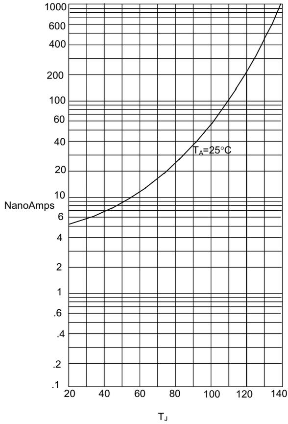
Instantaneous Reverse Leakage Current - NanoAmperes versus
