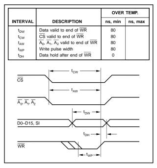
FIGURE 6. Logic Timing Diagram.
