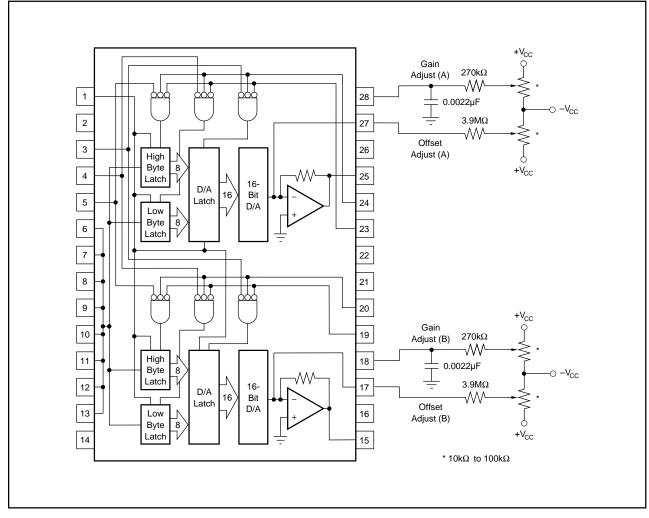
FIGURE 5. Connections for Gain and Offset Adjust.
