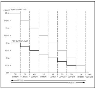
Figure 6. Output Fade DAC (Global Current = 0x07)
