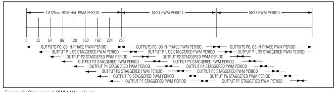
Figure 3. Staggered PWM Waveform
