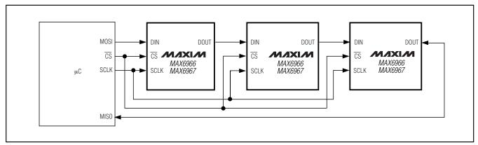
Figure 9. MAX6966/MAX6967 Daisy-Chain Connection
