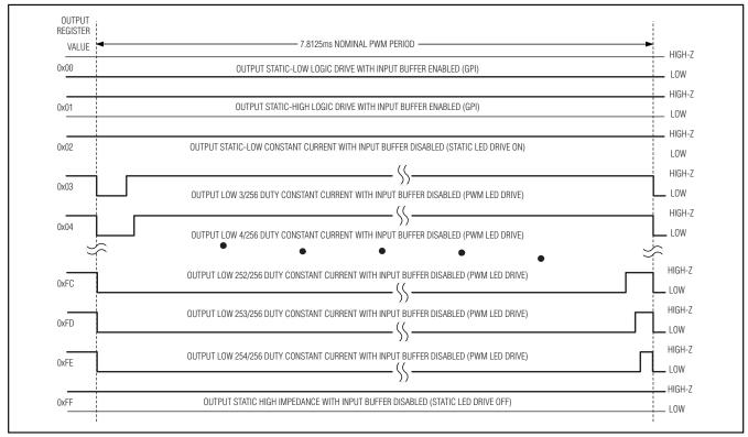
Figure 2. Static and PWM Constant-Current Waveforms
