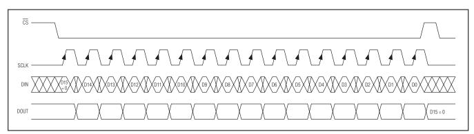
Figure 11. 16-Bit Write Transmission to the MAX6966/MAX6967
