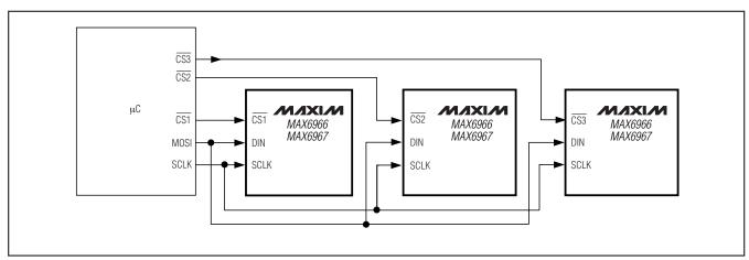
Figure 8. MAX6966/MAX6967 Multiple CS Connection
