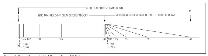
Figure 5. Ramp-Down, Hold-Off, and Fade-Off Behavior
