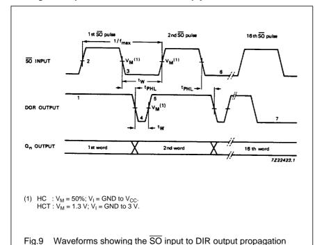
delay. The  $\overline{SO}$  pulse width and  $\overline{SO}$  maximum pulse frequency.
