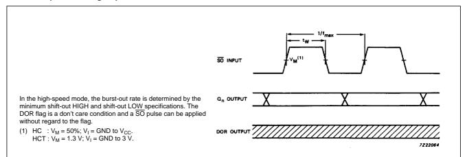
Fig.12 Waveforms showing SO minimum pulse width and maximum pulse frequency, in high-speed shift-out burst mode.
