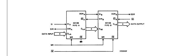
The PC7HC/HCT40105 is easily cascaded to increase word capacity without any external circuitry. In cascaded format, all necessary communications are handled by the FIFOs. Figs 17 and 19 demonstrate the intercommunication timing between FIFO<sub>A</sub> and FIFO<sub>B</sub>. Fig.22 gives an overview of pulse and timing of two cascaded FIFOs, when shifted full and shifted empty again.
