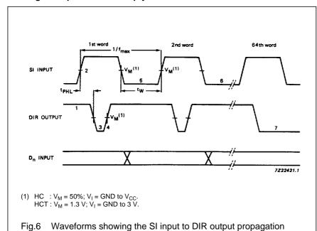
delay. The SI pulse width and SI maximum pulse frequency.
