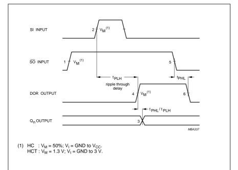
Fig.10 Waveforms showing ripple through delay SI input to DOR output and propagation delay from the DOR pulse to the Q<sub>n</sub> output.
