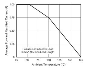
Fig. 1 - Forward Current Derating Curve
