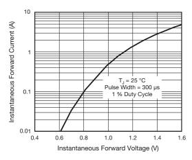
Fig. 3 - Typical Instantaneous Forward Characteristics
