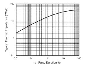
Fig. 6 - Typical Transient Thermal Impedance
