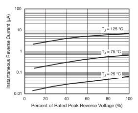
Fig. 4 - Typical Reverse Characteristics
