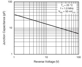
Fig. 5 - Typical Junction Capacitance
