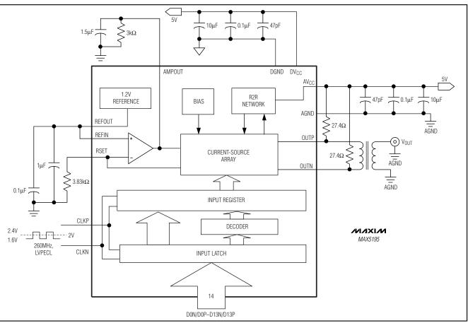
Figure 8. Decoupling and Bypassing Techniques for MAX5195—Typical Operating Circuit
