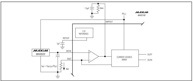
Figure 3. External Reference Configuration Using the MAX6520
