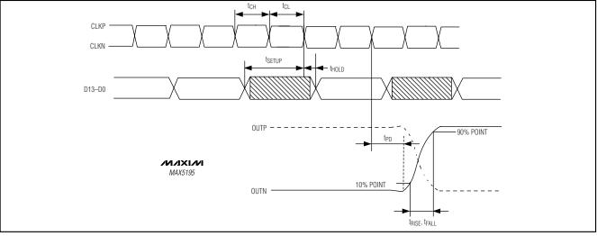
Figure 4. Input/Output Timing Information
