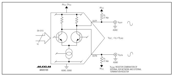
Figure 7a. Single-Ended Unbuffered Output Configuration
