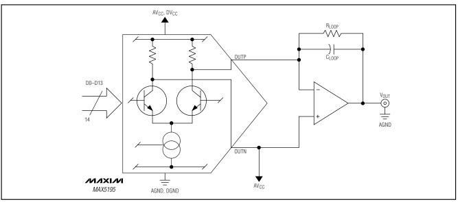
Figure 7b. Single-Ended Buffered Output Configuration
