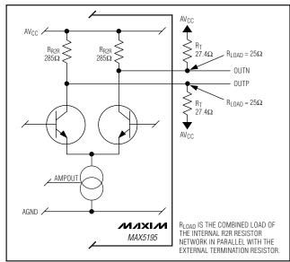
Figure 5. Simplified Output Architecture
