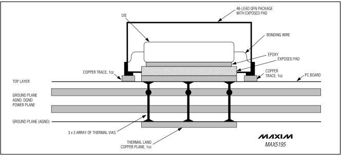
Figure 9. MAX5195 Exposed Paddle/PC Board Cross Section
