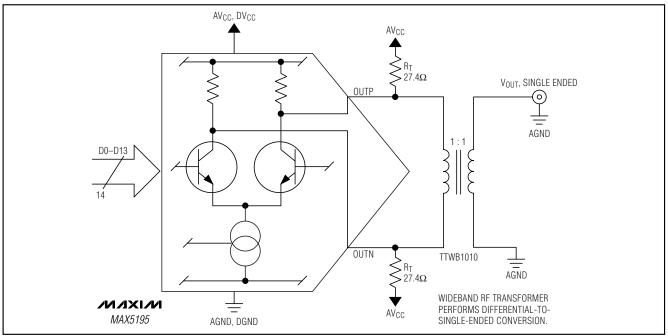
Figure 6. Differential Coupling Using a Wideband RF Transformer
