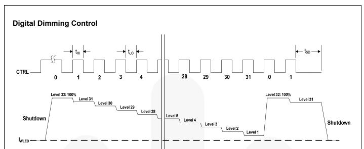
Figure 17. Digital Pulse Dimming Control Diagram
