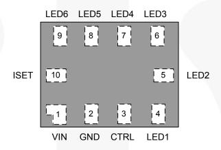
Figure 7. FAN5626: 10-Lead MicroPak™ MLP, Top View
