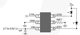
Figure 1. Typical Application of FAN5622
