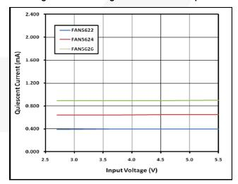
Figure 12. Shutdown Current vs. Input Voltage
