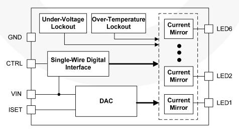
Figure 4. Block Diagram
