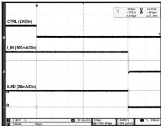
Figure 14. Startup Waveform for FAN5626
