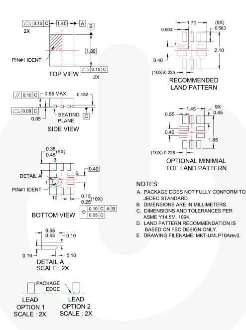
Figure 19. 10-Lead, Ultrathin Molded Leadless Package (UMLP)
