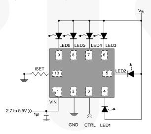
Figure 3. FAN5626 Typical Application for 6 LEDs
