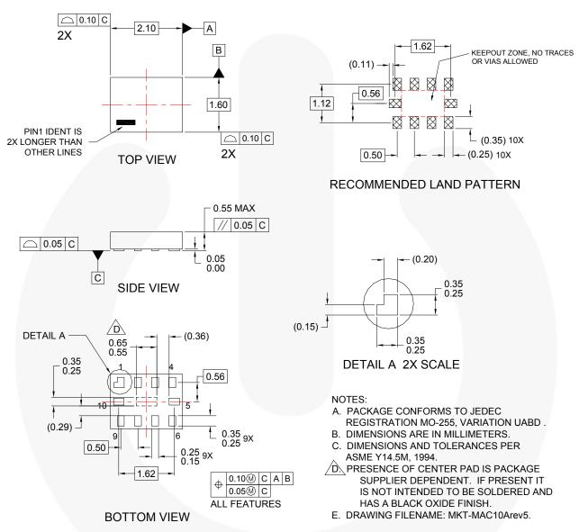
Figure 20. 10-Lead MicroPak™ MLP
