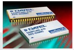
The ADS family of Sampling A/Ds combine a sample-hold and analog-to-digital converter with support circuitry, in a single-packaged device.
