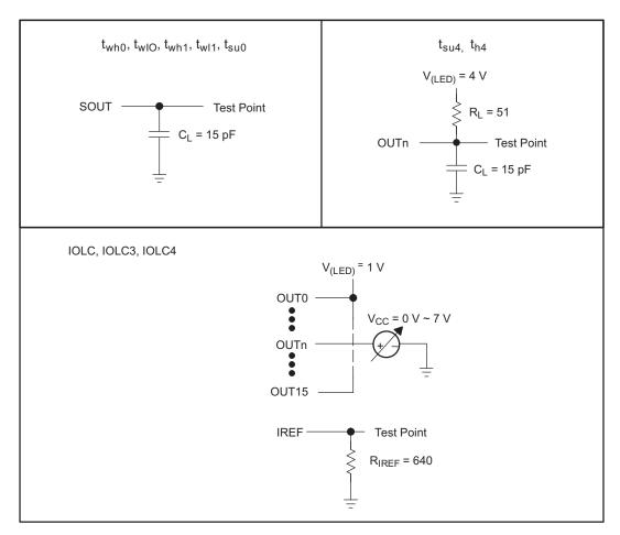
Figure 3. Parameter Measurement Circuits
