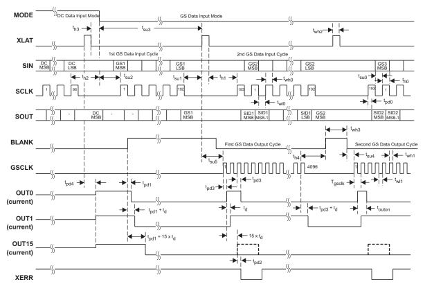
Figure 12. Serial Data Input Timing Chart
