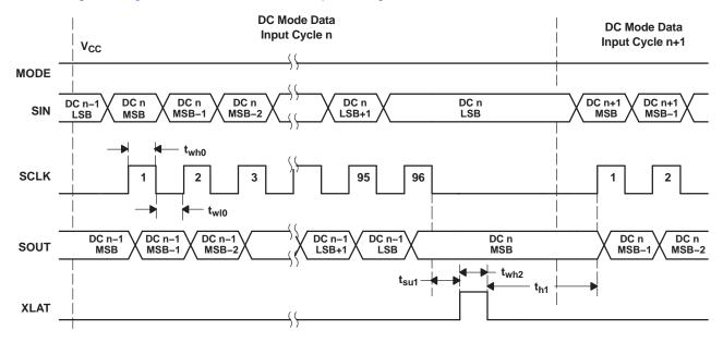
Figure 16. Dot Correction Data Input Timing Chart
