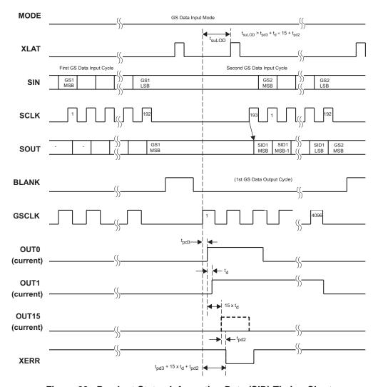
Figure 20. Readout Status Information Data (SID) Timing Chart
