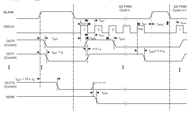
Figure 21. Grayscale PWM Cycle Timing Chart
