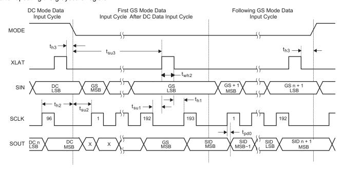
Figure 18. Grayscale Data Input Timing Chart
