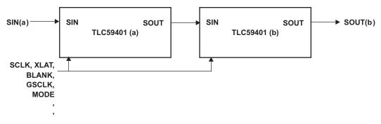
Figure 13. Cascading Two TLC59401 Devices
