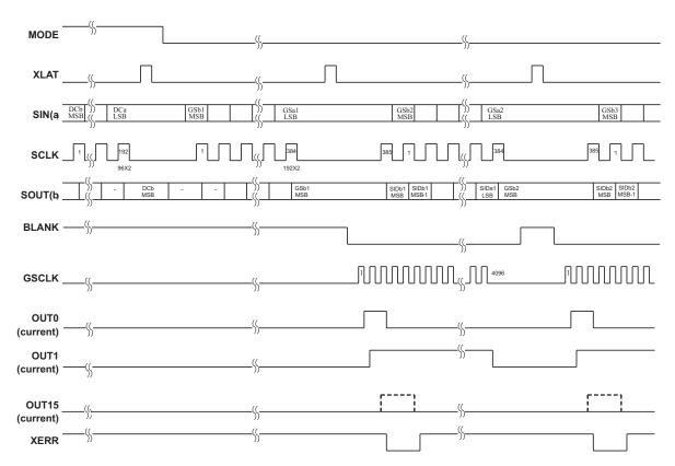
Figure 14. Timing Chart for Two Cascaded TLC59401 Devices
