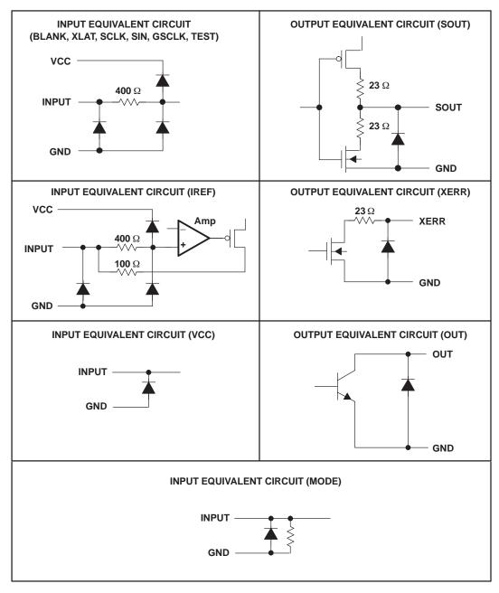
Figure 2. Input and Output Equivalent Circuits
