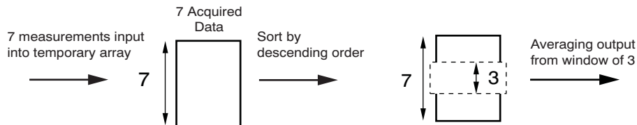
Figure 28. MAV Filter Operation (Patent Pending)
