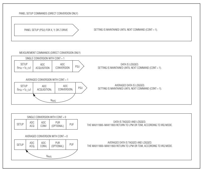
Figure 12. Panel Setup and Measurement Commands—MAX11800-MAX11803
