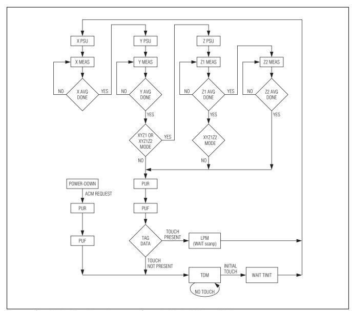
Figure 14. State Machine Transitions—Autonomous Conversion Mode—MAX11800/MAX11801
