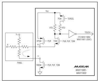
Figure 6. Touch-Detection Circuitry
