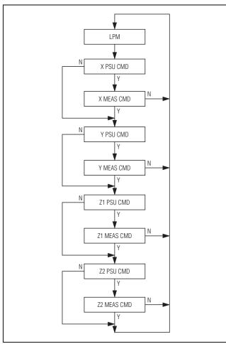
Figure 11. Command and Measurement Flow (DCM)
