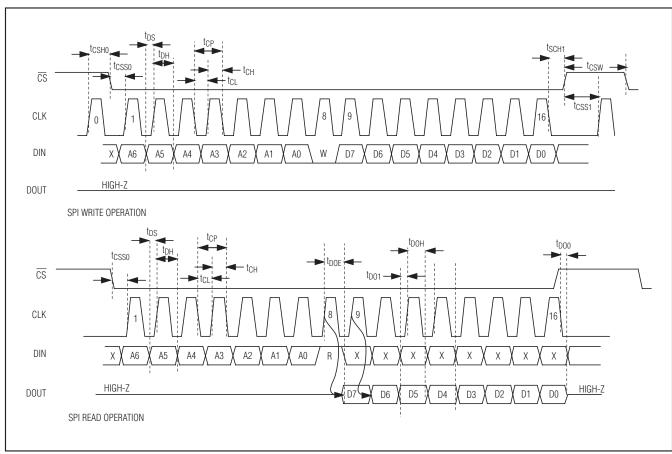
Figure 2. SPI Timing Diagram
