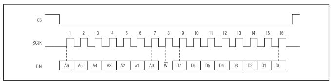
Figure 17. SPI Single Configuration Register Write Sequence—MAX11800/MAX11802
