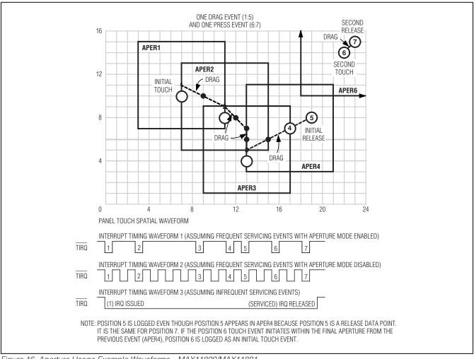
Figure 16. Aperture Usage Example Waveforms—MAX11800/MAX11801
