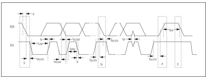
Figure 1. I<sup>2</sup>C Timing Diagram
