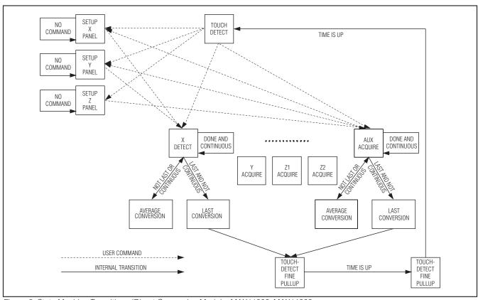
Figure 8. State Machine Transitions (Direct Conversion Mode)—MAX11800-MAX11803
