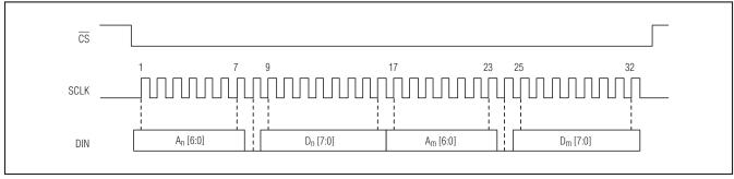
Figure 18. SPI Multiple Configuration Register Write Sequence—MAX11800/MAX11802
