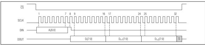
Figure 20. SPI Multiple-Byte Register Read Sequence—MAX11800/MAX11802
