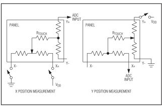
Figure 4. Position Measurements
