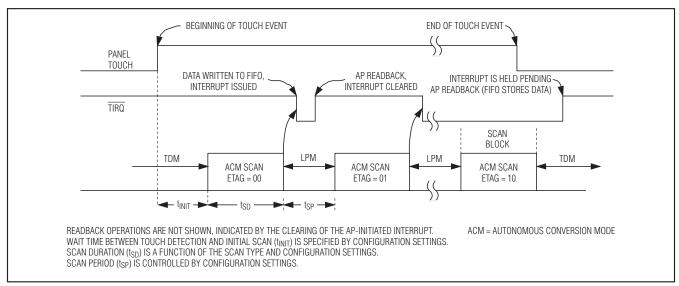
Figure 15. Clear-on-Read Interrupt Operation—MAX11800/MAX11801
