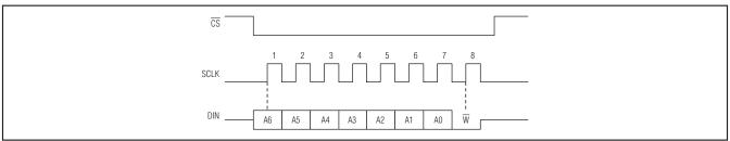
Figure 21. SPI Conversion Command—MAX11800/MAX11802
