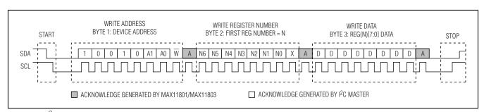
Figure 25. I<sup>2</sup>C Single Write Sequence
