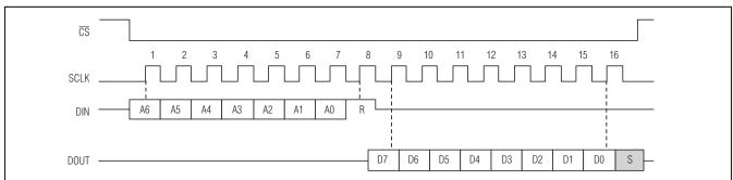
Figure 19. SPI Single-Byte Register Read Sequence—MAX11800/MAX11802
