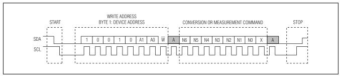
Figure 30. I<sup>2</sup>C Conversion and Measurement Commands
