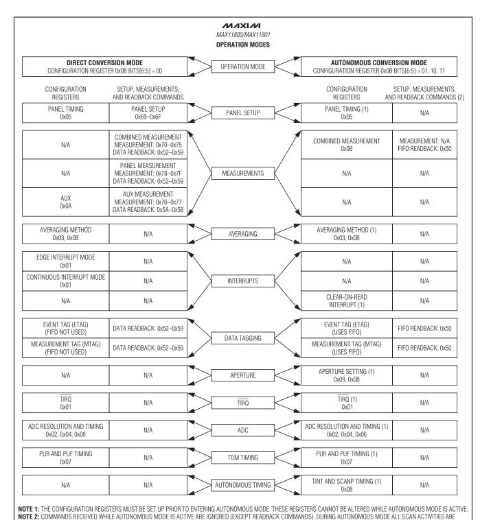
CONTROLLED BY THE MAX11800/MAX11801, BASED ON THE SETTINGS OF THE CONFIGURATION REGISTERS. ALL MEASUREMENT RESULTS ARE STORED IN THE ON-CHIP FIFO.
