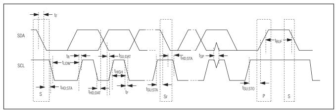
Figure 22. 2-Wire Interface Timing Diagram
