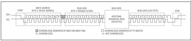
Figure 29. I<sup>2</sup>C Streamlined Read Sequence
