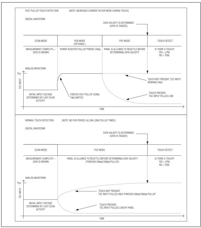
Figure 7. Touch-Detection Operations
