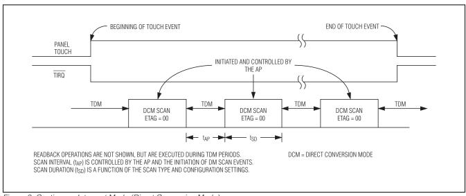
Figure 9. Continuous Interrupt Mode (Direct Conversion Mode)
