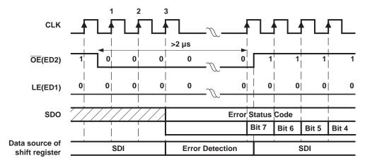
Figure 19. Reading Error Status Code
