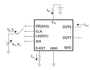
Figure 6. Test Circuit for Electrical Characteristics
