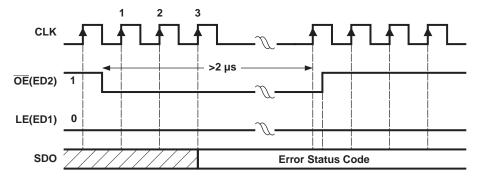
Figure 4. Reading Error Status Code
