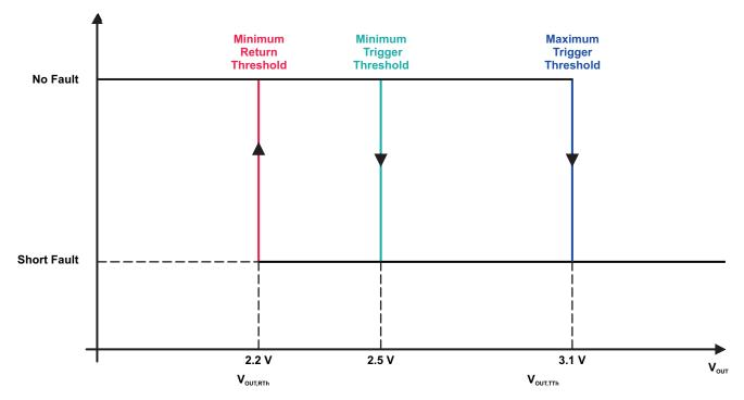
Figure 21. Short-Circuit Detection Principle
