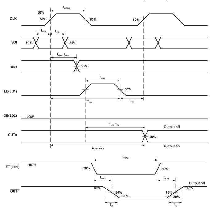
Figure 8. Normal Mode Timing Waveforms
