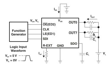
Figure 7. Test Circuit for Switching Characteristics
