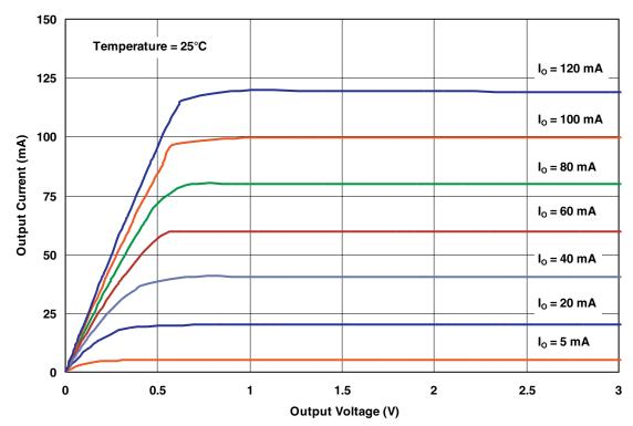
Figure 14. Output Current vs Output Voltage
