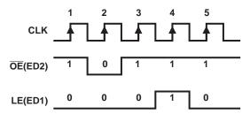
Figure 2. Switching to Special Mode
