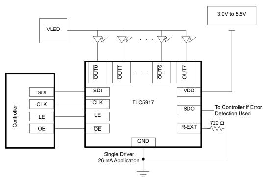
Figure 16. Single Implementation of TLC5916/TLC5917 Device
