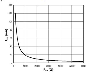
Figure 15. Default Relationship Curve Between I<sub>OUT,target</sub> and R<sub>ext</sub> After Power Up
