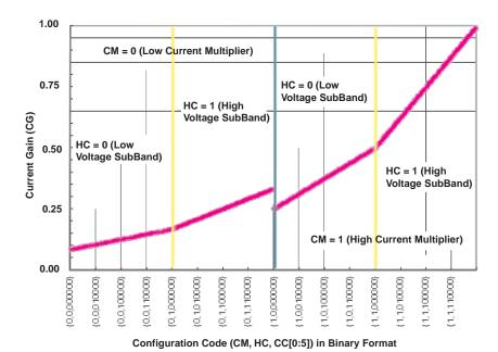
Figure 22. Current Gain vs Configuration Code
