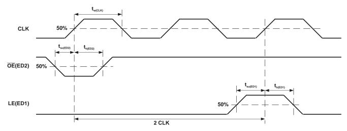
Figure 9. Switching to Special Mode Timing Waveforms
