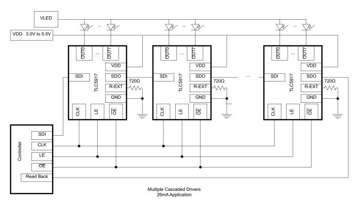
Figure 17. Cascading Implementation of TLC5916/TLC5917 Device
