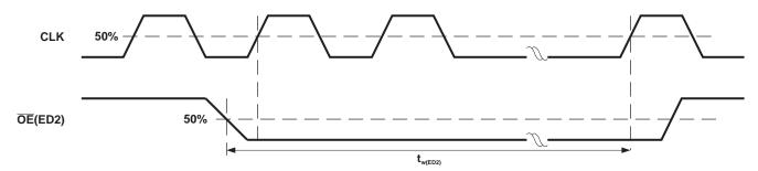
Figure 10. Reading Error Status Code Timing Waveforms
