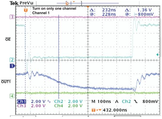
Figure 12. Response Time,  $\overline{\text{OE}}$  to  $\overline{\text{OUT1}}$
