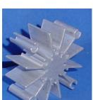
Wakefield's new 882 series heat sinks can be used with LEDs in the star package from Lumileds, Osram, and others. The radial design and fin area is ideally suited for natural convection applications such as ceiling lighting. A fan can also be used for increased performance in a forced convection application. Three sets of mounting holes allow maximum flexibility.
