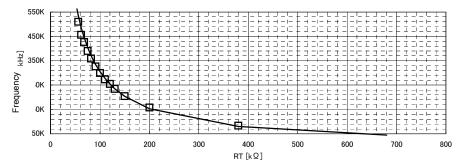
Fig.15 RT versus switching frequency
