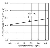
Fig.4 ILED temperature characteristic
