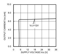
Fig.9 Circuit Current (Switching OFF)
