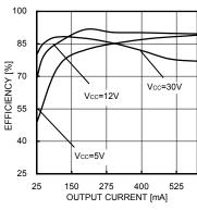
Fig.7 Efficiency (Depend on input voltage)
