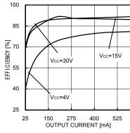
Fig.8 Efficiency (Depend on output voltage)
