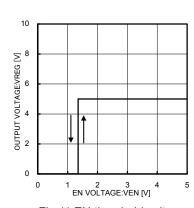
Fig.11 EN threshold voltage
