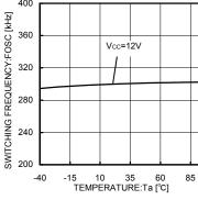
Fig.2 OSC temperature characteristic
