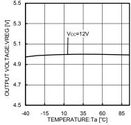
Fig.1 VREG temperature characteristic
