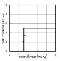
Fig.12 PWM threshold voltage
