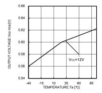
Fig.10 Overcurrent detecting voltage temperature characteristic
