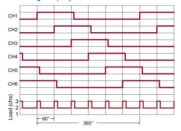
Phased dimming reduces the transient load on the boost converter, minimizing supply current ripple. This in turn, reduces conducted EMI on the supply rail and minimizes possible interference to adjacent circuitry. It also effectively sextuples the PWM dimming frequency, allowing a low PWM dimming frequency for dynamic range, while extending the audible effects beyond the range of human hearing.
