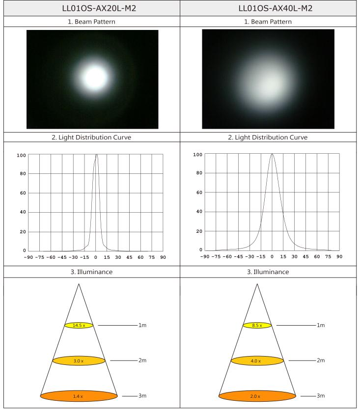
Notes: The Flux of Osram W5AM LED is 80 Im
