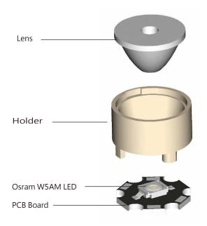
2. View assembly lens with MCPCB:
