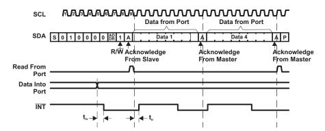
Figure 12. Read From Input Port Register
