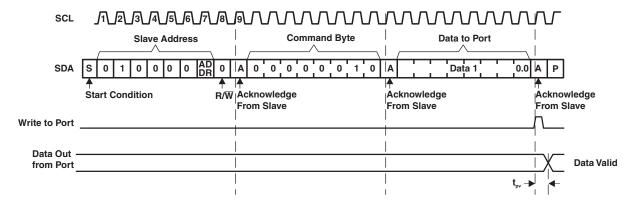
Figure 9. Write to Output Port Register
