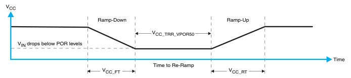
Figure 2. V<sub>CC</sub> is Lowered Below the POR Threshold, Then Ramped Back Up to V<sub>CC</sub>
