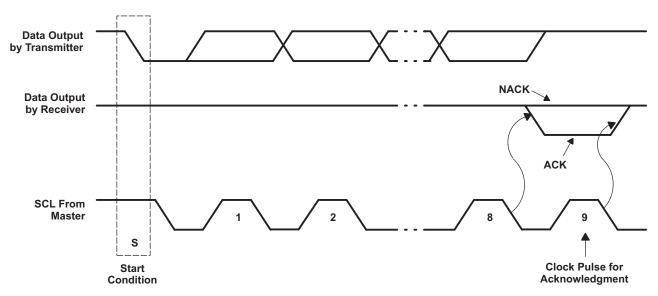
Figure 7. Acknowledgment on the I<sup>2</sup>C Bus
