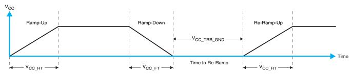
Figure 1. V<sub>CC</sub> is Lowered Below 0.2 V or 0 V and Then Ramped Up to V<sub>CC</sub>
