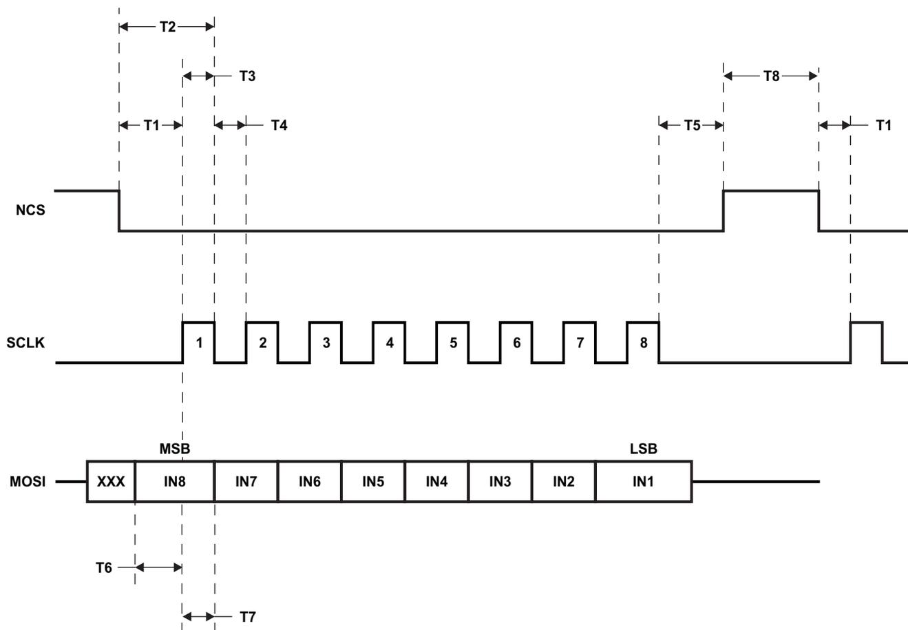
Figure 1. Serial Communications
