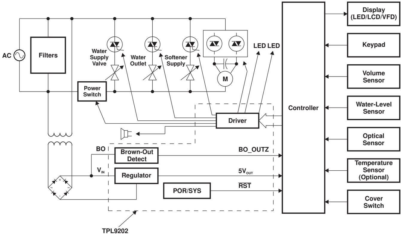
**Figure 3. Washing-Machine Application**
