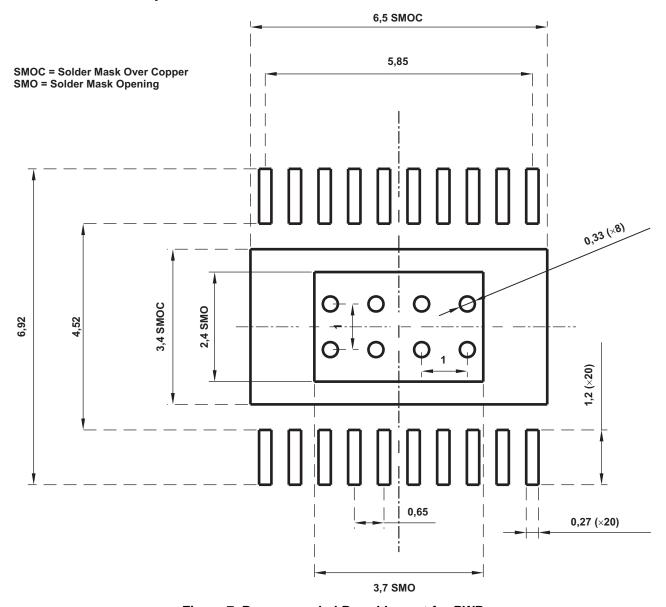
Figure 7. Recommended Board Layout for PWP
