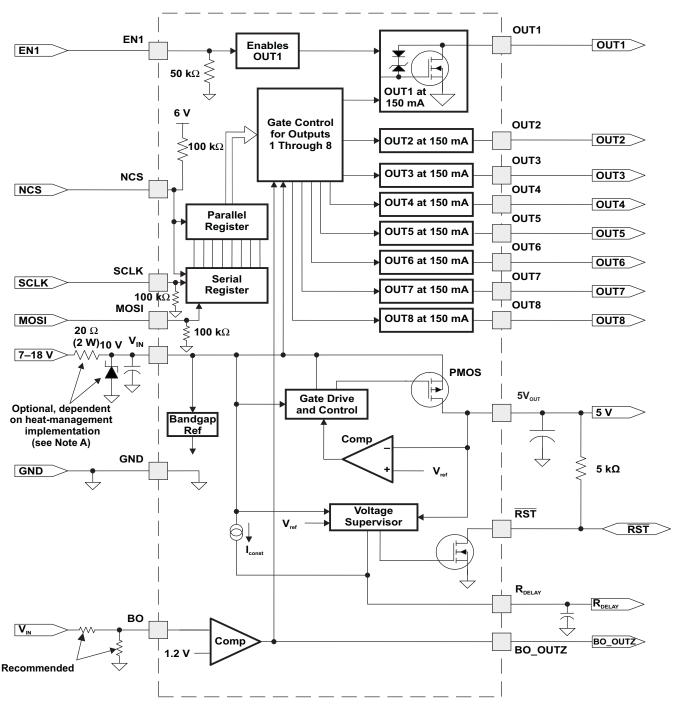
A. The resistor and Zener diode are required if there is insufficient thermal-management allocation.
