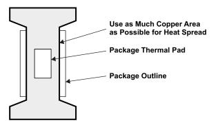
Figure 6. Layout Recommendations for a Single-Layer PCB
