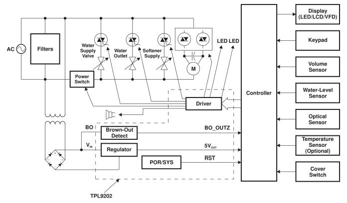
Figure 3. Washing-Machine Application
