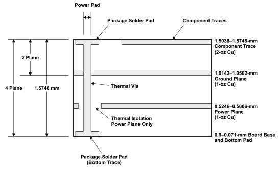
Figure 5. Multilayer Board (Side View)
