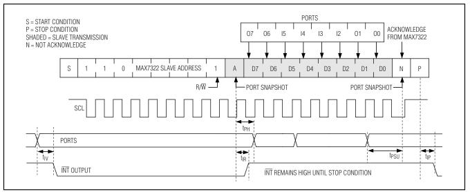
Figure 6. Reading from the MAX7322 (1 Data Byte)
