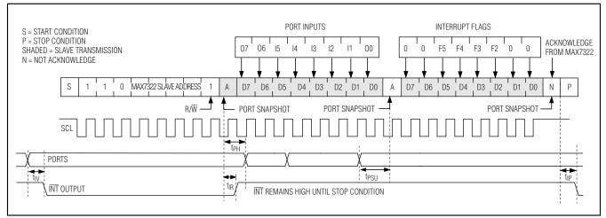
Figure 7. Reading from the MAX7322 (2 Data Bytes)
