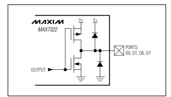
Figure 9. MAX7322 Push-Pull Output Port Structure
