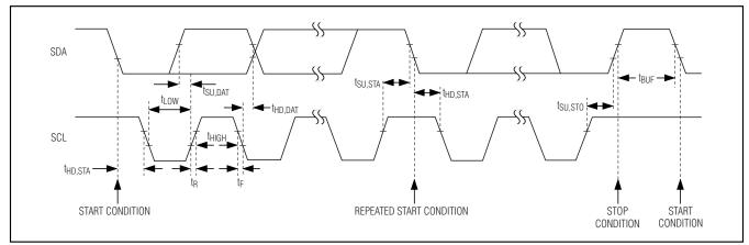
Figure 1. 2-Wire Serial Interface Timing Details
