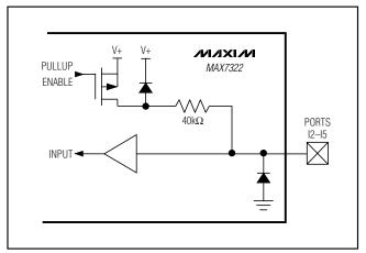
Figure 10. MAX7322 Input Port Structure
