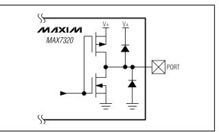
Figure 8. Output Port Structure
