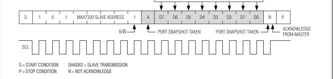
Figure 6. Reading the MAX7320
