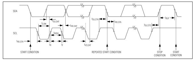
Figure 1. 2-Wire Serial-Interface Timing Details
