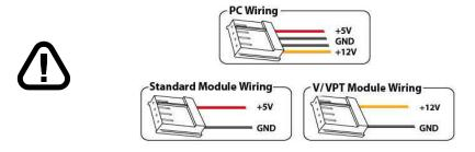
Figure 10: PC vs Matrix Orbital Display Module Wiring
