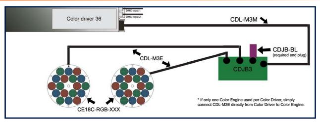
CDL-M3E is equipped with 8 individual colored wires. Each wire to be soldered onto indicated solder pad on color engine. For CE3C-RGB, cut off brown and purple leads.
