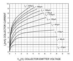
Figure 1. Static Characteristic
