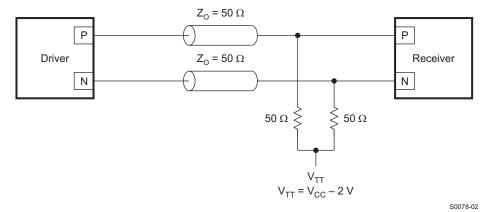
Figure 1. Typical Termination for Output Driver
