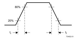
Figure 3. Output Rise and Fall Times
