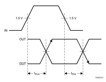
Figure 2. Output Propagation Delay
