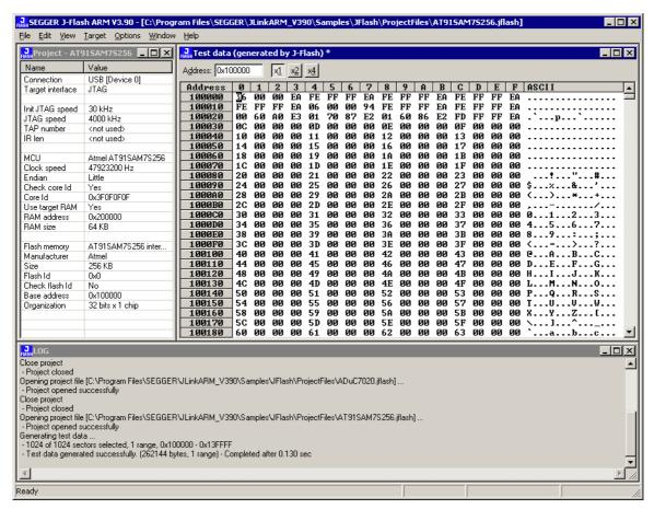
Before downloading the configuration (project) and program data (data file) to Flasher ARM, the connection type (USB/IP) needs to be selected in the project. These settings are also saved on a per-project basis, so this also only needs to be setup once per J-Flash project. The connection dialog is opened by clicking Options -> Project settings -> General.
