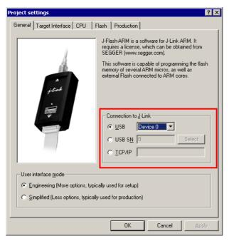
The connection dialog allows the user to select how to connect to Flasher ARM. When connecting to a Flasher via TCP/IP it is not mandatory to enter an IP address. If the field is left blank and <code>File->Download</code> to <code>programmer</code> is selected, an emulator selection dialog pops up which shows all Flasher which have been found on the network. The user then can simply select the Flash he wants to download the configuration to.
