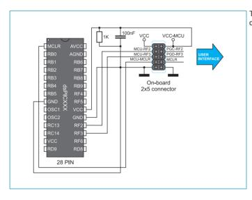
The connection schematic for 2x5 male connector and 28-pin dsPIC30F microcontrollers such as dsPIC30F2012, 3013 etc.
