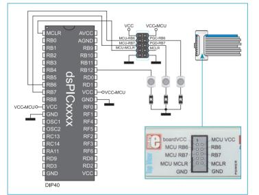
Figure 1-3: Microcontroller and 2x5 connector connection
