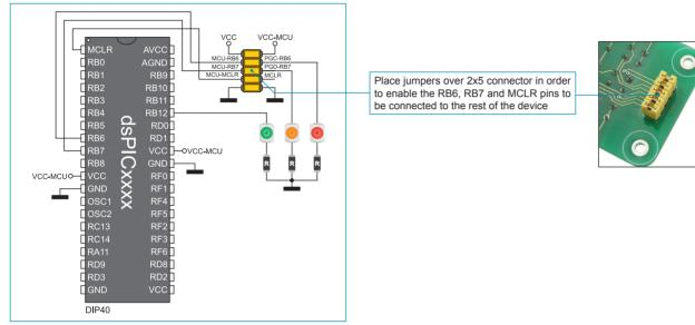
Figure 4-1: Microcontroller after programming
