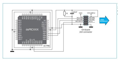
The connection schematic for 2x5 male connector and 44-pin dsPIC30F microcontrollers such as dsPIC30F3014, 4013 etc.
