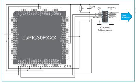
The connection schematic for 2x5 male connector and 64-pin dsPIC30F microcontrollers such as dsPIC30F6014, 5013 etc.
