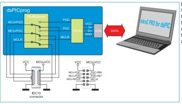
**Figure 2-2:** The multiplexer in the operating mode. When the programming process has been completed, the multiplexer releases the microcontroller pins used for programming, thus enabling them to be used as inputs/outputs. This also enables the programmer to remain connected to the target device without affecting its operation.
