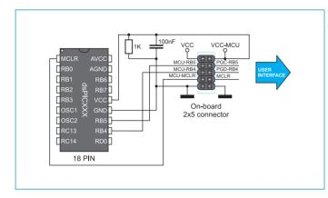
The connection schematic for 2x5 connector and 18-pin dsPIC30F microcontrollers such as dsPIC30F3012, 2011 etc.
