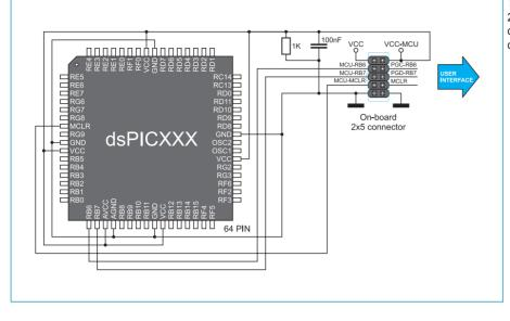
The connection schematic for 2x5 male connector and 64-pin dsPIC30F microcontrollers such as dsPIC30F5015, 5011 etc.
