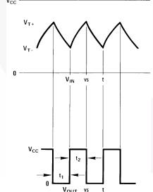
$$f \approx \frac{1}{\text{RC In} \frac{V_{T+}(V_{CC} - V_{T-})}{V_{T-}(V_{CC} - V_{T+})}}$$
