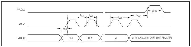
Figure 11. VFD Interface Timing Diagram
