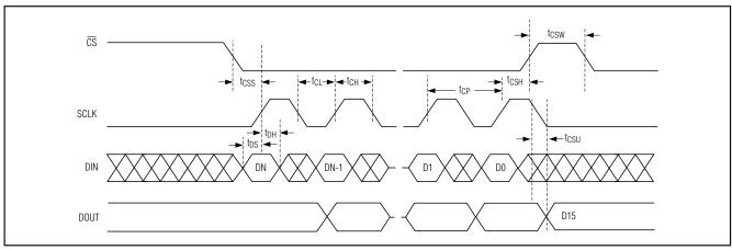
Figure 8. 4-Wire Serial Interface Timing Diagram
