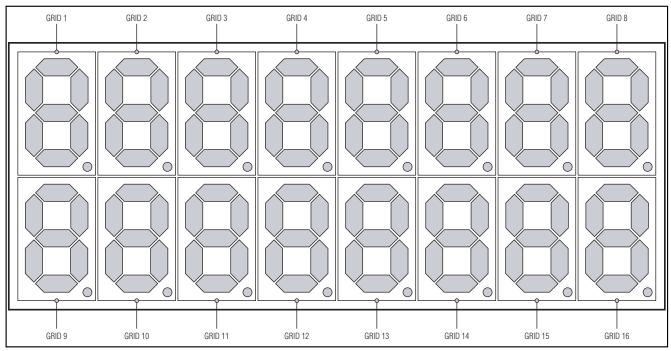
Figure 1. Example of a One-Digit-per-Grid Display
