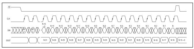
Figure 10. Transmission of More than 16 Bits to the MAX6850
