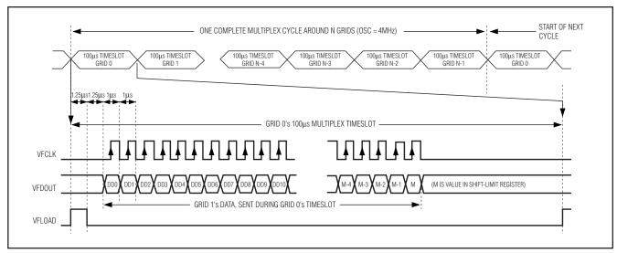
Figure 12. VFD Multiplex Timing Diagram
