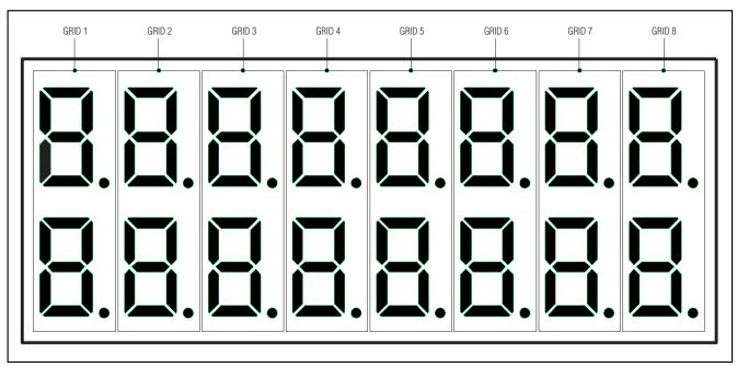
Figure 2. Example of a Two-Digit-per-Grid Display
