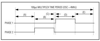
Figure 14. Filament Bridge Driver Timing Waveforms
