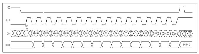
Figure 9. 16-Bit Write Transmission to the MAX6850
