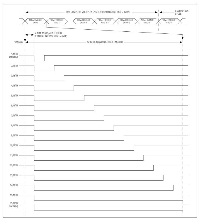
Figure 13. BLANK and Intensity Timing Diagram
