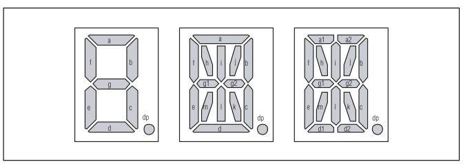
Figure 5. Segment Labeling for 7-, 14-, and 16-Segment Displays
