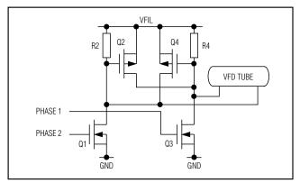
Figure 15. Filament Bridge Driver (MOSFET)
