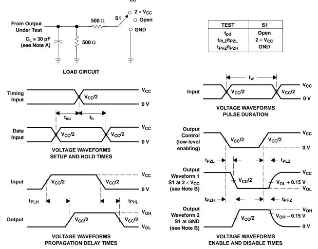
NOTES: A. C<sub>1</sub> includes probe and jig capacitance.
