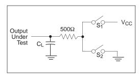
Figure 4. Driver Timing Test Load #2 Circuit
