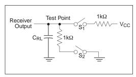
Figure 2. Receiver Timing Test Load Circuit
