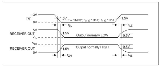
Figure 8. Receiver Enable and Disable Times
