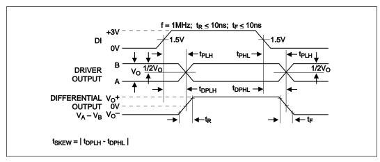
Figure 5. Driver Propagation Delays
