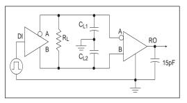
Figure 3. Driver/Receiver Timing Test Circuit
