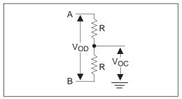
Figure 1. Driver DC Test Load Circuit
