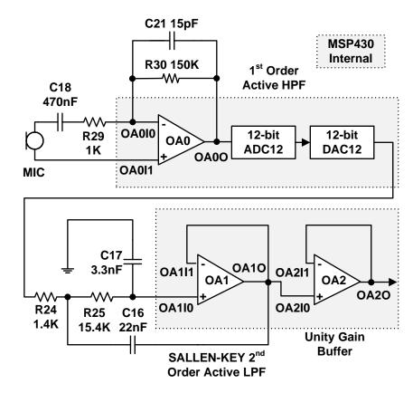
Figure 5: Active Analog Filter setup
