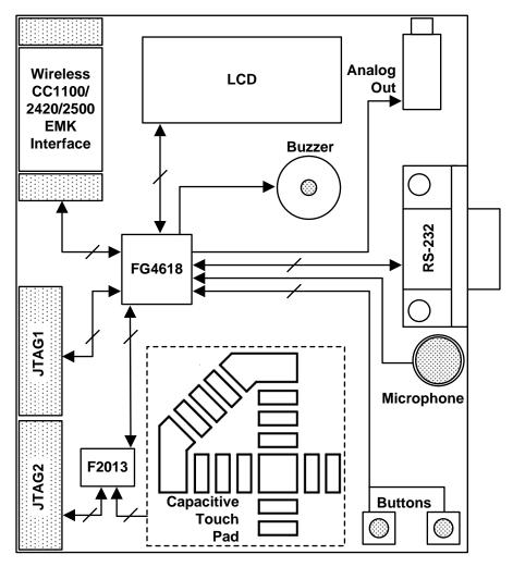
Figure 2: Experimenter's Board Block Diagram
