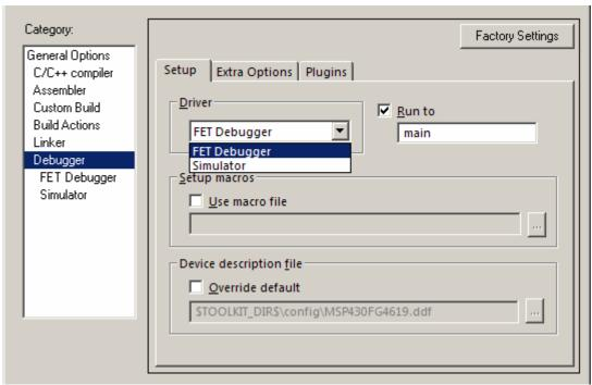
Figure A-2: Selecting the FET Debugger
