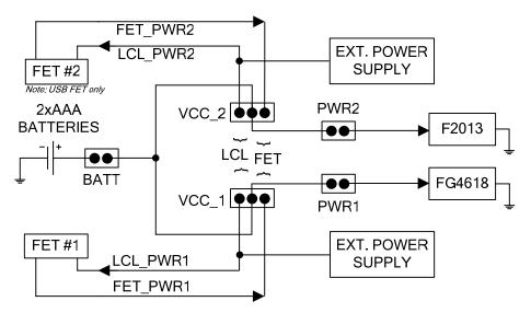
Figure 3: Jumper Settings for Power Selection
