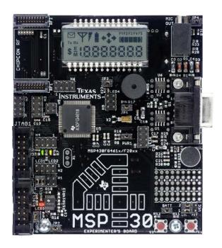
Figure 1: MSP430FG4618/F2013 Experimenter's Board
