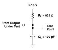
Figure 4. Test Load Circuit
