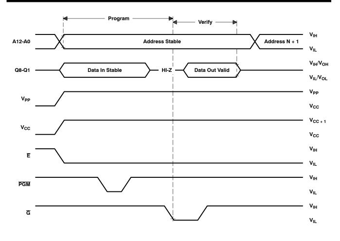
Figure 11. Fast Programming Timing
