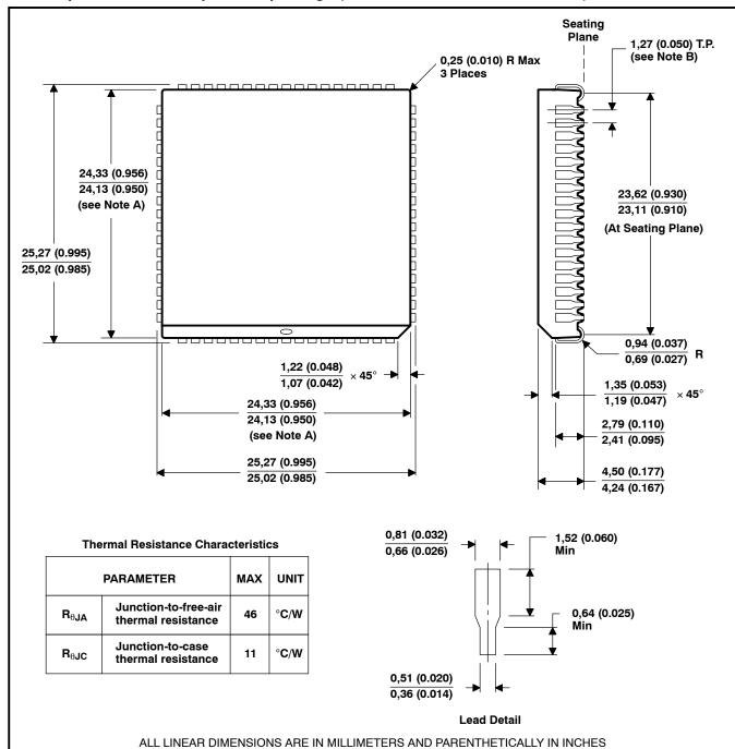
68-lead plastic leaded chip carrier package (TMS320C25 and TMS320C25-50)
