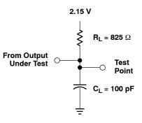
Figure 3. Test Load Circuit
