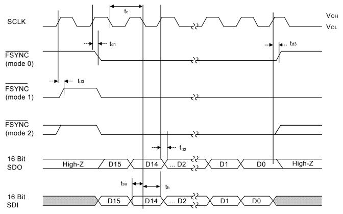
Figure 2. Serial Interface Timing Diagram
