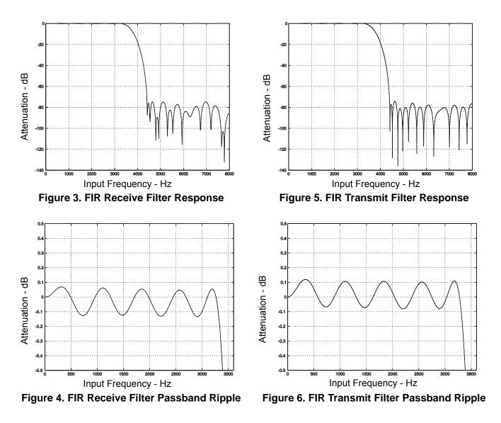
For Figures 3–6, all filter plots apply to a sample rate of Fs = 8 kHz. The filters scale with the sample rate as follows:
