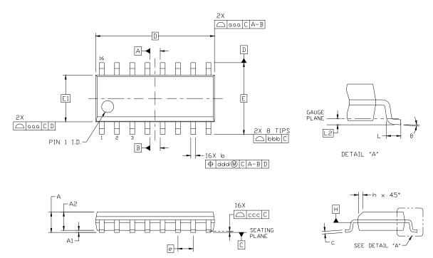
Figure 19. 16-Pin Small Outline Integrated Circuit (SOIC) Package
