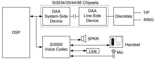
Figure 14. Si3000 with Silicon Labs DAA System Diagram
