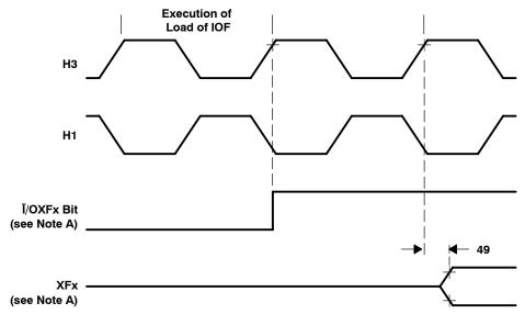
NOTE A: Ī/OXFx represents either bit 1 or bit 5 of the IOF register, and INXFx represents either bit 3 or bit 7 of the IOF register depending on whether XF0 or XF1, respectively, is being affected.
