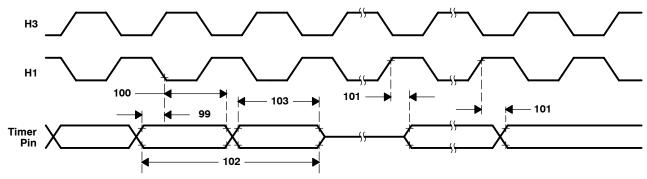
NOTE A: Period and polarity of valid logic level are specified by contents of internal control registers.
