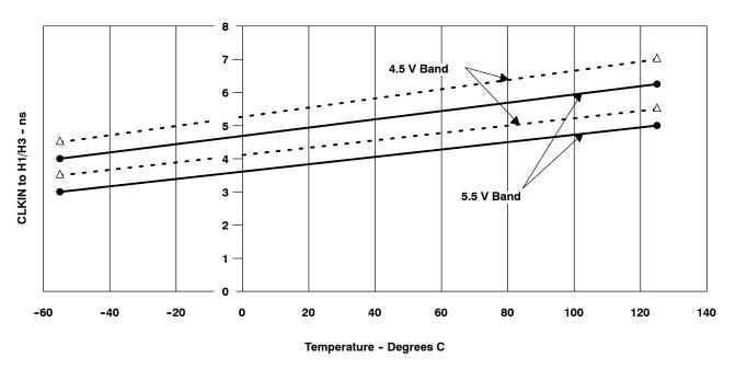
Figure 9. CLKIN to H1/H3 as a Function of Temperature (Typical)
