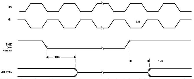
NOTE A: Enabling SHZ destroys SMJ320C30 register and memory contents. Assert SHZ and reset the SMJ320C30 to restore it to a known condition.
