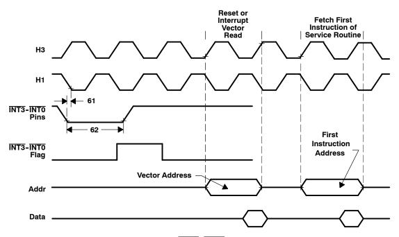
Figure 21. Timing for INT3-INT0 Response [Q=t<sub>c(H)</sub>]
