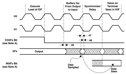
NOTE A: Ī/OXFx represents either bit 1 or bit 5 of the IOF register, and INXFx represents either bit 3 or bit 7 of the IOF register depending on whether XF0 or XF1, respectively, is being affected.
