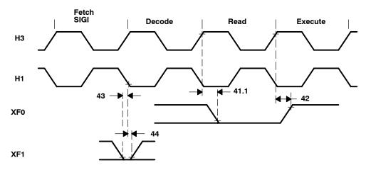
Figure 16. Timing for XF0 and XF1 When Executing SIGI
