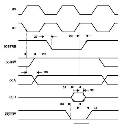
Figure 12. Timing for Memory (IOSTRB = 0) Read
