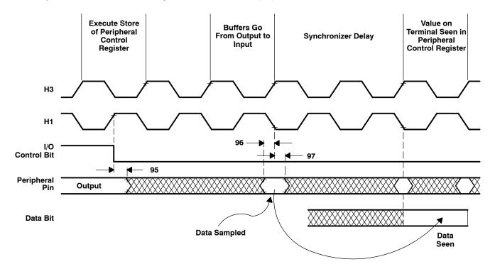
Figure 27. Timing for Change of Peripheral Pin From General-Purpose Output to Input Mode
