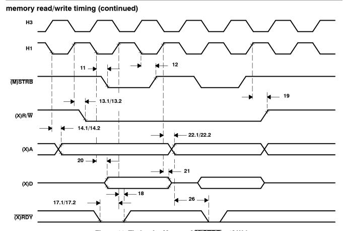
Figure 11. Timing for Memory  $[(\overline{M})\overline{STRB} = 0]$  Write
