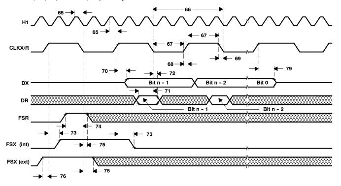
Figure 23. Serial-Port Timing for Fixed-Data-Rate Mode
