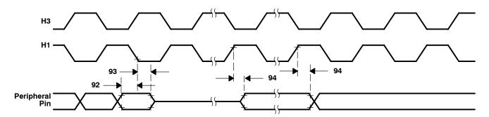
Figure 26. Timing for Peripheral Pin General-Purpose I/O
