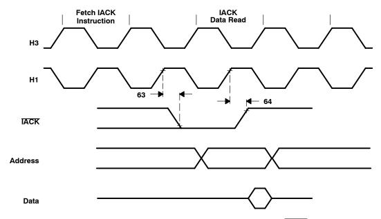
Figure 22. Timing for Interrupt-Acknowledge (IACK)
