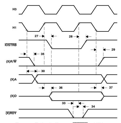
Figure 13. Timing for Memory (IOSTRB = 0) Write
