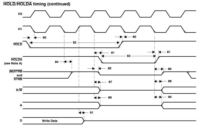
NOTE A: HOLDA goes low in response to HOLD going low and continues to remain low through one H1 cycle after HOLD returns to high.
