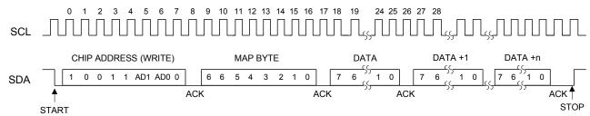
Figure 15. Control Port Timing, I2C Write
