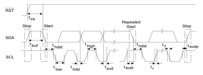
Figure 5. Control Port Timing - I<sup>2</sup>C Format
