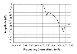
Figure 18. Single-Speed Stopband Rejection
