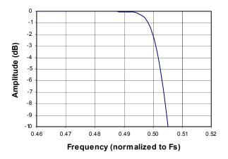
Figure 23. Double-Speed Transition Band (Detail)
