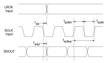
Figure 1. Master Mode Serial Audio Port Timing
