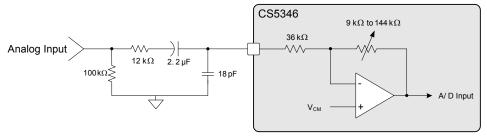
Figure 13. 2 V<sub>RMS</sub> Input Circuit
