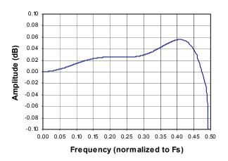
Figure 24. Double-Speed Passband Ripple
