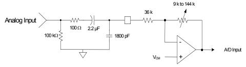
Figure 12. 1  $V_{RMS}$  Input Circuit with RF Filtering
