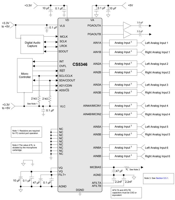
Figure 7. Typical Connection Diagram
