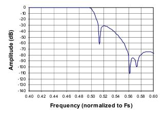
Figure 22. Double-Speed Stopband Rejection
