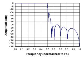
Figure 21. Double-Speed Stopband Rejection
