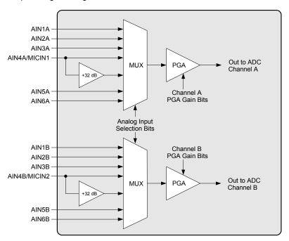
Figure 9. Analog Input Architecture
