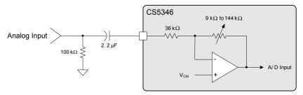
Figure 11. 1 V<sub>RMS</sub> Input Circuit
