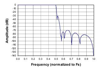
Figure 17. Single-Speed Stopband Rejection
