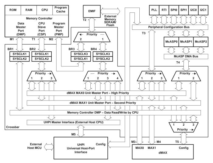
Figure 2-4. Block Diagram of Crossbar Switch
