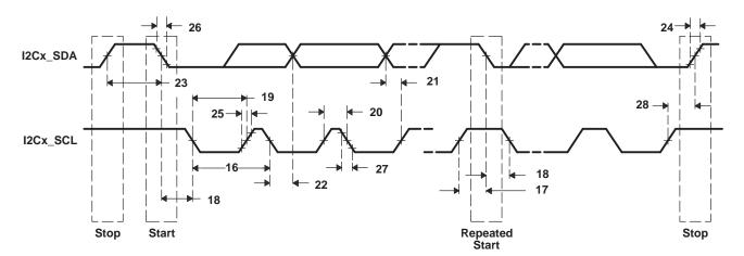
Figure 4-41. I2C Transmit Timings
