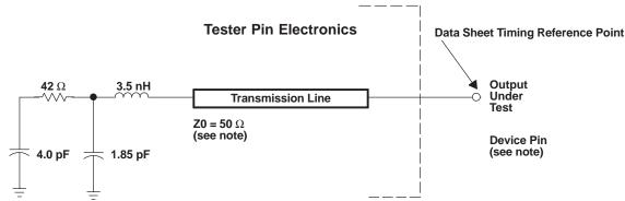
A. The data sheet provides timing at the device pin. For output timing analysis, the tester pin electronics and its transmission line effects must be taken into account. A transmission line with a delay of 2 ns or longer can be used to produce the desired transmission line effect. The transmission line is intended as a load only. It is not neccessary to add or subtract the transmission line delay (2 ns or longer) from the data sheet timings.
