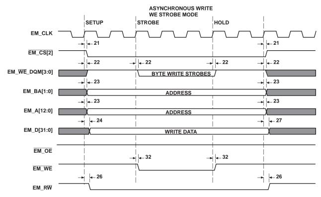
Figure 4-13. Asynchronous Write WE Strobe Mode
