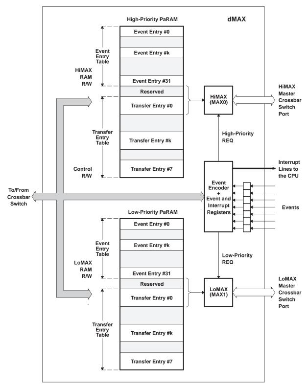
Figure 4-6. dMAX Controller Block Diagram
