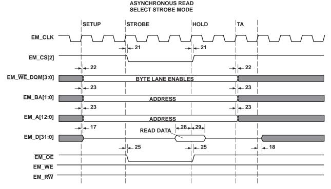
Figure 4-12. Asynchronous Read Select Strobe Mode
