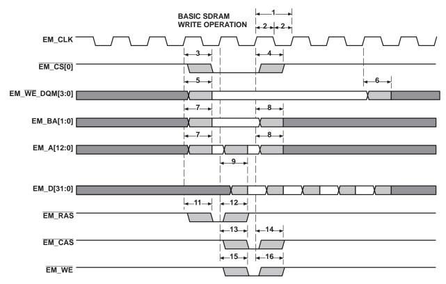
Figure 4-9. Basic SDRAM Write Operation
