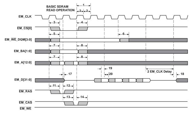
Figure 4-10. Basic SDRAM Read Operation
