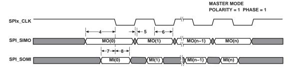
Figure 4-35. SPI Timings—Master Mode
