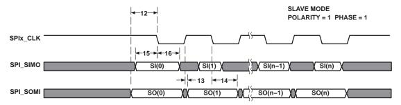
Figure 4-36. SPI Timings—Slave Mode
