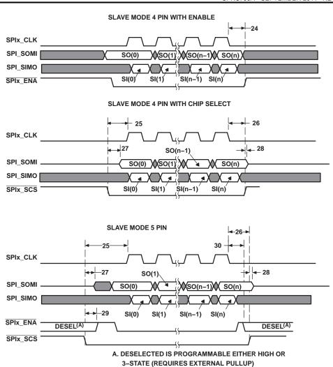
Figure 4-38. SPI Timings—Slave Mode (4-Pin and 5-Pin)
