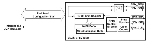
Figure 4-33. Block Diagram of SPI Module
