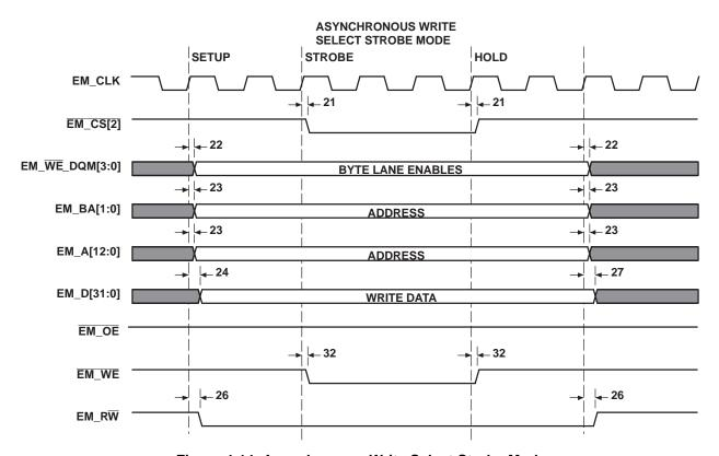
Figure 4-14. Asynchronous Write Select Strobe Mode
