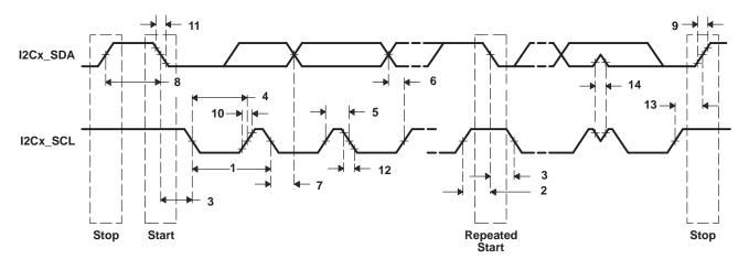
Figure 4-40. I2C Receive Timings
