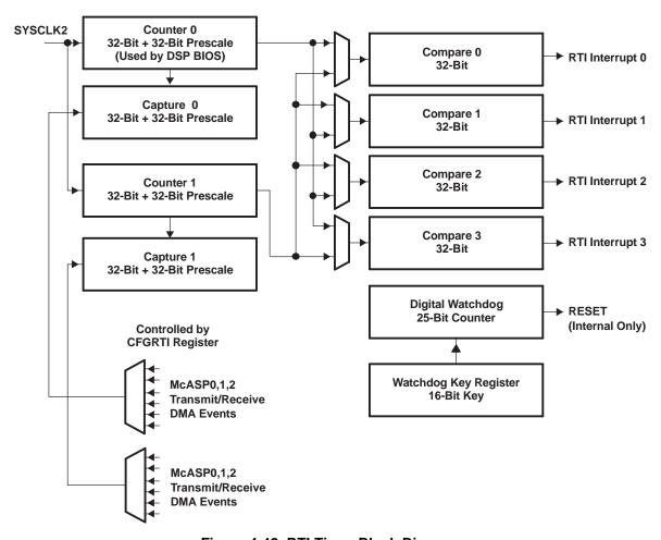
Figure 4-42. RTI Timer Block Diagram
