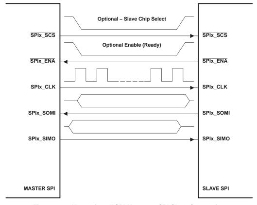
Figure 4-34. Illustration of SPI Master-to-SPI Slave Connection
