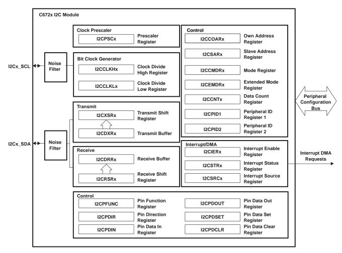
Figure 4-39. I2C Module Block Diagram
