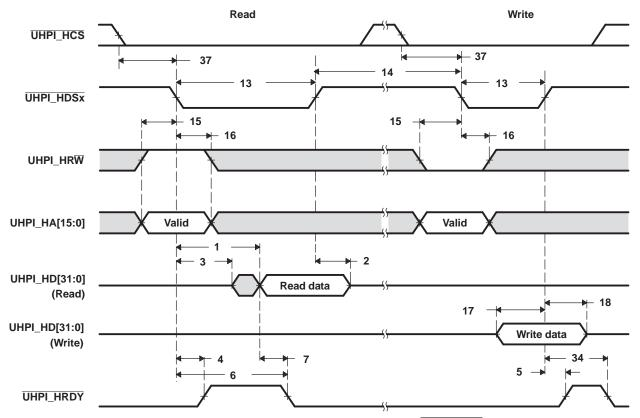
A. Depending on the type of write or read operation (HPID or HPIC), transitions on UHPI\_HRDY may or may not occur.
