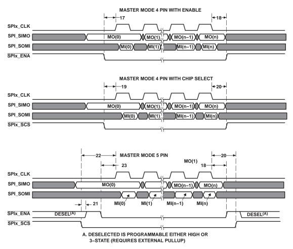
Figure 4-37. SPI Timings—Master Mode (4-Pin and 5-Pin)
