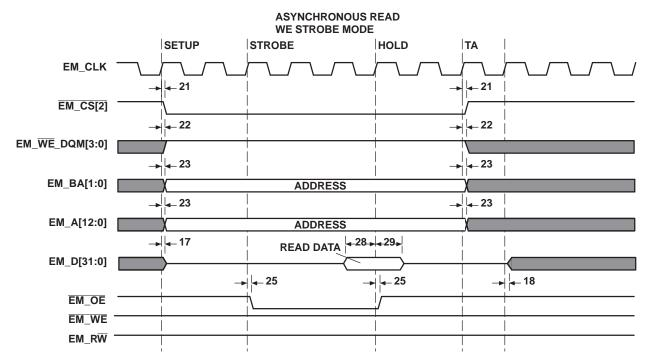
Figure 4-11. Asynchronous Read WE Strobe Mode
