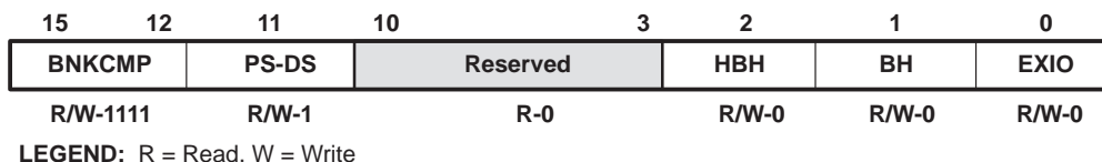
Figure 6. Bank-Switching Control Register (BSCR), MMR Address 0029h
