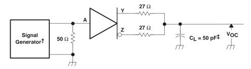
$^{\dagger}$  PRR = 1 MHz, 50% duty cycle,  $t_{f}$  < 6 ns,  $t_{f}$  < 6 ns, Z\_{O} = 50  $\Omega$   $^{\ddagger}$  Includes probe and jig capacitance
