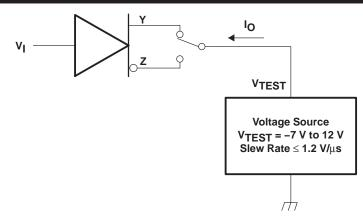
Figure 7. Test Circuit, Short-Circuit Output Current
