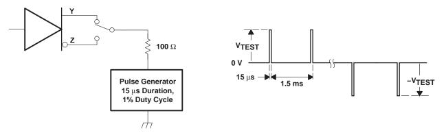
Figure 8. Test Circuit and Waveform, Transient Over-Voltage
