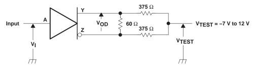
Figure 2. Test Circuit, V<sub>OD</sub> With Common-Mode Loading
