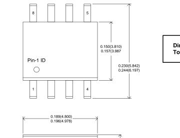
Dimensions are in milimeters(inches). Top line: (MIN) and Bottom line: (Max)
