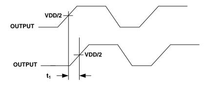
Figure 1. Output to Output Skew
