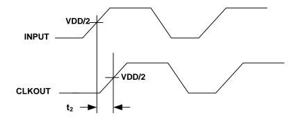
Figure 2. Input to Output Skew
